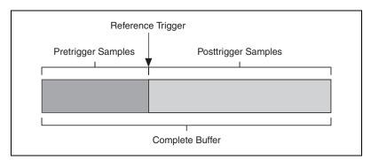
Figure 4-14. Reference Trigger Final Buffer
